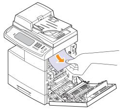
If the jammed paper is inside the fuser, remove the jammed paper in the direction show.
